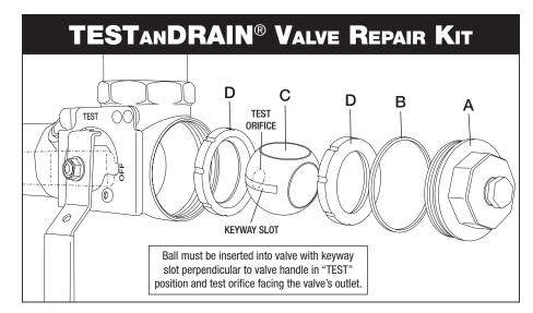
Repair Kit Includes: (1) adapter gasket (B), (1) ball (C), (2) valve seats (D), (1) stem packing (not shown, see Note 1) and (1) stem washer (not shown, see Note 1).
