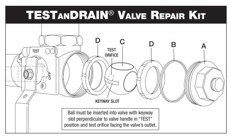
Repair Kit Includes: (1) adapter gasket (B), (1) ball (C), (2) valve seats (D), (1) stem packing (not shown, see Note 1) and (1) stem washer (not shown, see Note 1).
